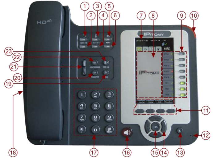
Figure 4 IPitomy IP620 Buttons and Hardware Definitions
