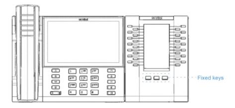
The Mitel M695 PKM features a 4.3" 480x272 pixel color backlit LCD display that provides a unified graphical user experience with the Mitel MiVoice 6940 IP phone.
