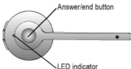
3. Dock the new headset in the base. The new headset is paired with the base after 1 minute.
