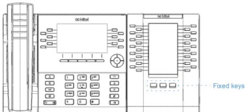
The Mitel M695 PKM features a 4.3" 480x272 pixel color backlit LCD display that provides a unified graphical user experience with the Mitel MiVoice 6930 IP phone.
